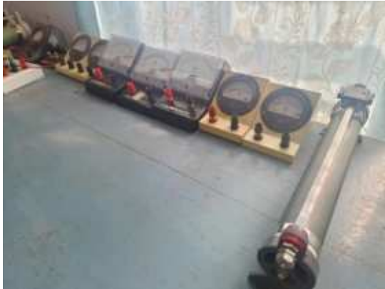
MAYERS OSCILLATING DISC SET UP
